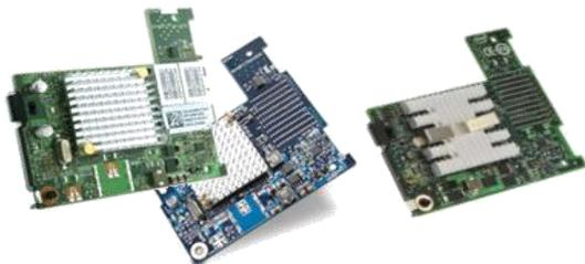
Combine the 10Gb Pass-Through with **Broadcom 57710 / 57711** or **Intel X520-x/k** dual-port 10Gb mezzanine cards for 10Gb Ethernet from server to LAN switch
