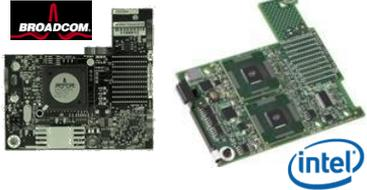
Use Broadcom 5709 or Intel Gigabit Ethernet mezzanine cards or Fabric A LOMs in PE blade servers for Gigabit Ethernet I/O connectivity
