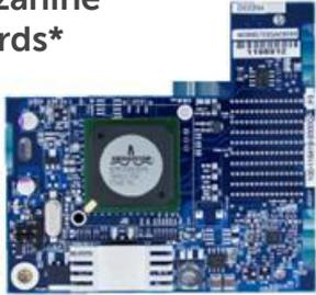
Use Broadcom 5709 dual port **server blade I/O Mezzanine Cards** in PE blade servers for Gigabit Ethernet I/O connectivity
