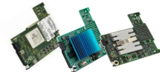
Combine the 10Gb Pass-Through with **QLogic QME8142**, **Emulex OCm10102-f-m**, or **Intel X520-x/k** converged network adapters to the top-of-rack FCoE-enabled switch of your choice
