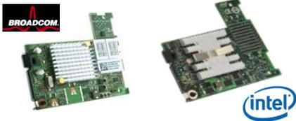
Combine the 10Gb M8024 Ethernet switch with the **Broadcom 57710/57711** or **Intel X520-x/k** dual-port 10Gb Ethernet mezz cards in PE blade servers for 10Gb from server to LAN
