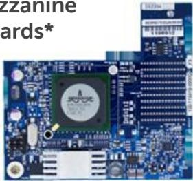
Use Broadcom 5709 dual port server blade I/O Mezzanine Cards or Gigabit LOMs in PE blade servers for Gigabit Ethernet I/O connectivity
