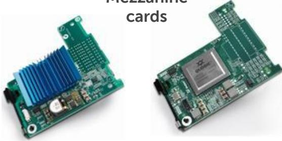
Combine the M5424 with the **Qlogic QME2572 or Emulex LPe1205 Server Blade I/O Mezzanine Card** in PE blade servers for end-to-end 8Gbps I/O. FC4 mezz cards are also supported with this switch at 4Gbps.
